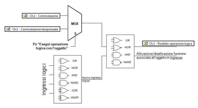
it can be used to enable the execution of the commands received by the BUS on the Ch. x - Switching,
