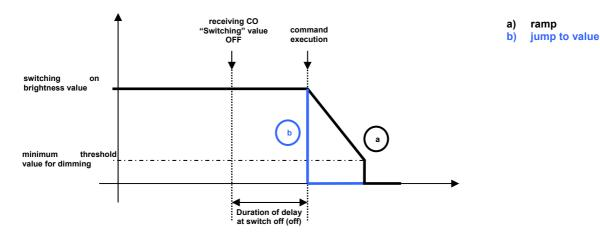
If selecting the double step value, the switching off phase is divided into two steps. When an off command is received, the jump to value 0% (0) or the start of a down ramp are delayed by 50% of the value defined by the parameter "**Duration of delay at switch OFF**". The brightness value is changed (jump or ramp) to 50% of the "Switching ON brightness value" and maintained for the remaining 50% of the time. When the delay has expired, the brightness value is changed to 0% (jump or ramp).
