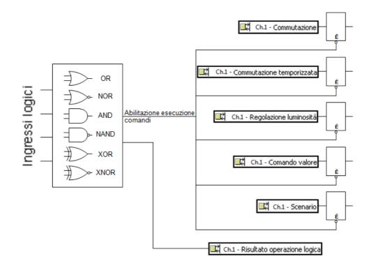
The parameter used to select the function of the outcome of the operation between logic inputs is "The outcome of the operation between logic inputs stands for" that, in the case of a single logic input, is replaced by the parameter "The logic input value stands for". These parameters can assume the following values:
