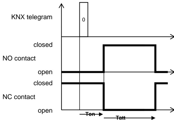
Selecting “**1**” value, when the device receives a telegram from the BUS with a logic value equal to “1”, after the set activation delay time ( $T_{on}$ ) has passed it switches the relay to the status → NO contact closed/NC contact open. See figure below.
