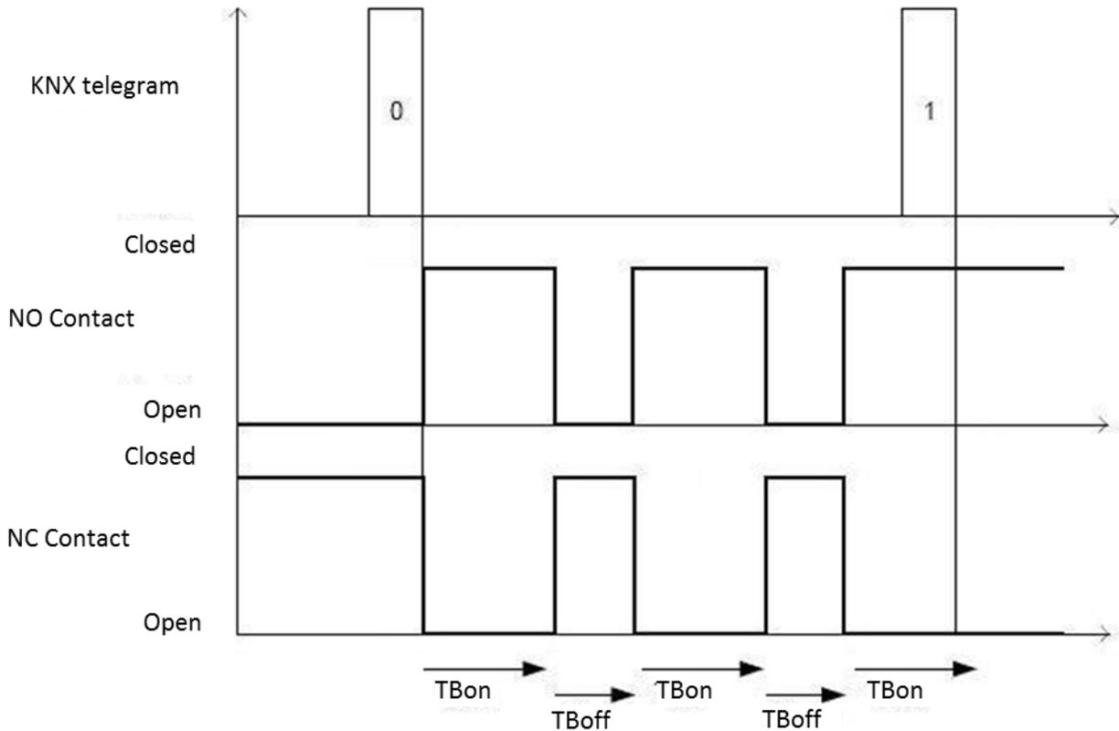
If you select **value "1"**, then when the device receives a telegram from the BUS with a logic value equal to "1", it switches the relay to the status → NO contact closed/NC contact open, and begins the activation time count; At the end of the activation time, the device deactivates the load (NO contact open/NC contact closed) for a period of time equal to the deactivation time, and then reactivates the load and restarts the process. See the following figure for more information.
