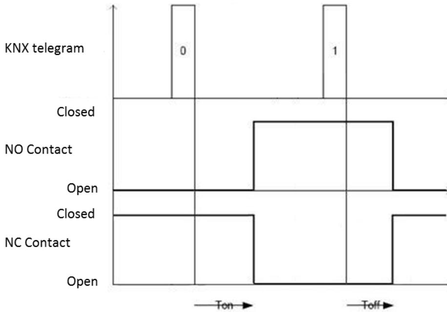
Selecting **value “1”**, when the device receives a telegram from the BUS with a logic value equal to “1”, after the set activation delay time (Ton) has passed it switches the relay to the status → NO contact closed/NC contact open; Vice versa, when the logic value “0” is received, the device waits for the deactivation delay time (Toff) before switching the contact to → NO contact open/NC contact closed. See figure below.
