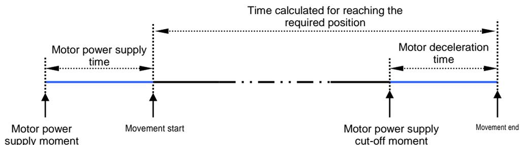
NOTE: the times set for the “*Motor start time*” and “*Motor deceleration time*” parameters are only used to calculate the time required to reach a certain intermediate percentage position (following a specific command, or following the reproduction of a position associated with a scene or prior to a status). They are not used for any movements carried out via the **Ch.y/z - Movement** object.
