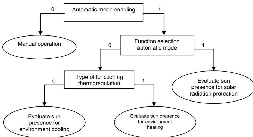
For the various types of control (temperature adjustment or solar radiation protection), you can therefore define the behaviour of the device according to whether it is sunny or not.
