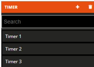
To remove a timer from the list, just activate the context menu of the object and select the “Delete” command. You can even eliminate all the timers simultaneously by pressing the
