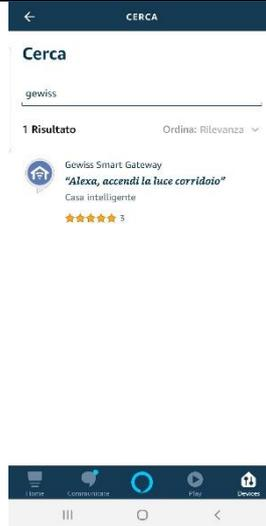
Once Skill Gewiss is selected, the Smart Gateway authentication page opens. Enter the access credentials used to access the Smart gateway portal/app.
