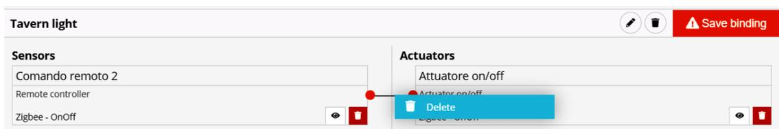
After clicking “Delete”, the “Save connection” push-button turns orange. Clicking it removes the binding (unbind). the push-button turns green to indicate that the operation was successful.
