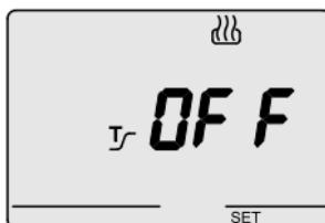
The time-thermostat manages the advance automatically, so as to guarantee the set temperature at the beginning of every period of the programmed profile.
