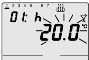
Press the MODE key for 5 seconds to activate the function: the symbol is displayed on the VDU and the set point value active at that time starts to blink.
