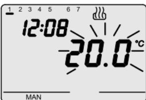
To activate manual operating mode the MODE key is pressed until the message "MAN" is displayed on the VDU. The temperature set point begins to blink for about 2 seconds. The **▲▼** keys are used to set the required set point value. Press the MODE key or wait 5 seconds to confirm the setting.
