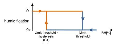
When the reference relative humidity is lower than value C1 (Limit threshold-hysteresis"), the device sends the command associated with Condition 1; when the reference relative humidity reaches value C2 (Limit threshold), the device sends the command associated with Condition 2.
