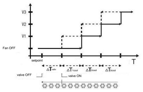
The figure shows fan coil speed control with three operating stages and two-point fan coil valve management (**ON-OFF** or **0-100%**) with regards cooling. The charts shows that each stage has a hysteresis cycle, and each speed is associated with two thresholds that determine its activation and deactivation. The thresholds are determined by the values set for the various regulation differentials, and can be summarised as follows:
