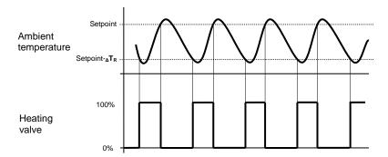
When the measured temperature is lower than the value "setpoint- $\Delta T_R$ " (where  $\Delta T_R$  identifies the value of the heating regulation differential), the device activates the heating system by sending the relative BUS percentage command to the actuator that manages it. When the measured temperature reaches the defined setpoint value, the device deactivates the heating system by sending the relative BUS percentage command to the actuator that manages it.
