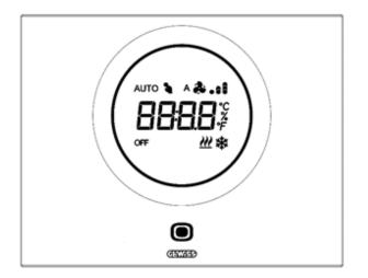
In simplified operating mode, the icons for the active HVAC mode are disabled with both HVAC mode and setpoint control.
