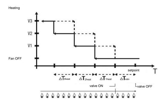
The figure shows fan coil speed control with three operating stages and two-point fan coil valve management (**ON-OFF** or **0-100%**) with regards heating. The charts shows that each stage has a hysteresis cycle, and each speed is associated with two thresholds that determine its activation and deactivation.
