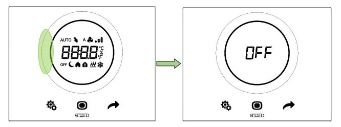
To reactivate the signal in stand-by, repeat the procedure; in this case, the word "On" will appear.
