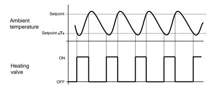
When the measured temperature is lower than the value "setpoint- $\Delta T_R$ " (where  $\Delta T_R$  identifies the value of the heating regulation differential), the device activates the heating system by sending the relative BUS command to the actuator that manages it. When the measured temperature reaches the defined setpoint value, the device deactivates the heating system by sending the relative BUS command to the actuator that manages it.
