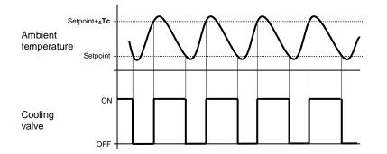
When the measured temperature is higher than the value "setpoint+ $\Delta Tc$ " (where  $\Delta Tc$  identifies the cooling regulation differential), the device activates the cooling system by sending the relative BUS command to the actuator that manages it. When the measured temperature reaches the defined setpoint value, the device deactivates the cooling system by sending the relative BUS command to the actuator that manages it.
