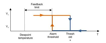
When the measured temperature falls below the **Alarm threshold**, the device can be configured to send a command; another command can be sent when the measured temperature exceeds the **Alarm threshold** value plus a **hysteresis** value.
