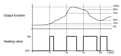
The device keeps the heating system switched on for a cycle time percentage that depends on the output function of the proportional-integral control; the device continuously regulates the heating system, modulating the system turning on-off times with a duty-cycle (shown to the right along the vertical axis) that depends on the output function value calculated at every time interval equal to the cycle time. The cycle time is reinitialised every time the reference set-point is modified.
