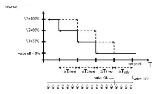
The figure refers to the control of the fancoil speeds with three operating stages for heating. The chart shows that each stage has a hysteresis cycle, and each speed is associated with two thresholds that determine the sending of the associated value. The thresholds are determined by values set for the various regulation differentials, and can be summarised as follows:
