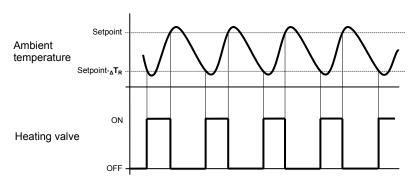
When the measured temperature is lower than the value setpoint- $_{\Delta}T_{R}$ " (where  $_{\Delta}T_{R}$  identifies the value of the heating regulation differential) the device turns on the heating system, sending the relative BUS command to the actuator that manages it; when the detected temperature reaches the fixed setpoint value, the device turns off the heating system, sending the relative BUS command to the BUS that manages it.
