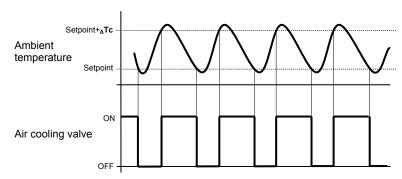
When the measured temperature is higher than the value "setpoint+  $_{\Delta}Tc$ " (where  $_{\Delta}Tc$  identifies the air cooling regulation differential) the device turns on the air cooling system, sending the relative BUS command to the actuator that manages it; when the detected temperature reaches the fixed setpoint value, the device turns off the air cooling system, sending the relative BUS command to the BUS that manages it.
