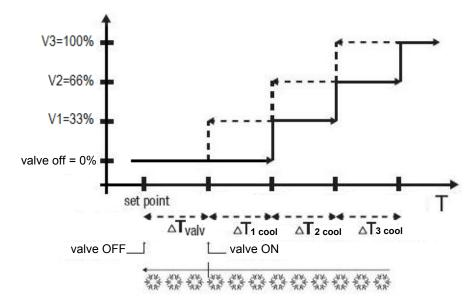
The figure below refers to the control of the speeds of a fancoil with three operating stages for air cooling. The chart shows that each stage has a hysteresis cycle, and each speed is associated with two thresholds that determine the sending of the associated value. The thresholds are determined by values set for the various regulation differentials, and can be summarised as follows:
