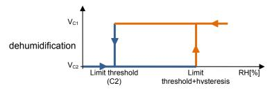
When the relative humidity of reference is higher than value C1 (limit threshold+hysteresis"), the device will sent the command associated with Condition 1; when the relative humidity of reference reaches value C2 (limit threshold), the device will sent the command associated with Condition 2,.
