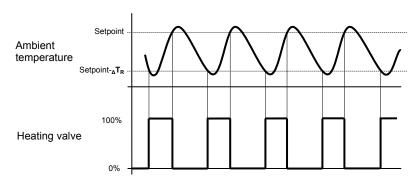
When the measured temperature is lower than the value setpoint- $_{\Delta}T_{R}$ " (where  $_{\Delta}T_{R}$  identifies the value of the heating regulation differential) the device turns on the heating system, sending the relative BUS percentage command to the actuator that manages it; when the detected temperature reaches the fixed setpoint value, the device turns off the heating system, sending the relative BUS percentage command to the BUS that manages it.
