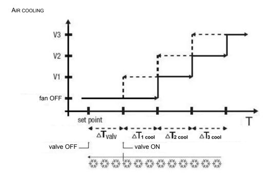
The figure refers to the control of the speeds of a fancoil with three operating stages for air cooling. The chart shows that each stage has a hysteresis cycle, and each speed is associated with two thresholds that determine its activation and deactivation. The thresholds are determined by values set for the various regulation differentials, and can be summarised as follows:
