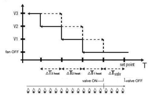
The figure refers to the control of the fancoil speeds with three operating stages for heating. The chart shows that each stage has a hysteresis cycle, and each speed is associated with two thresholds that determine its activation and deactivation. The thresholds are determined by values set for the various regulation differentials, and can be summarised as follows:
