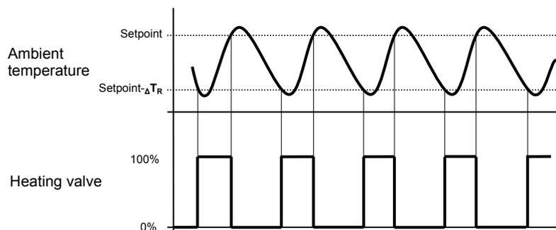
When the measured temperature is lower than the value setpoint- $\Delta T_R$ ” (where  $\Delta T_R$  identifies the value of the heating regulation differential) the device turns on the heating system, sending the relative BUS percentage command to the actuator that manages it; when the detected temperature reaches the fixed setpoint value, the device turns off the heating system, sending the relative BUS percentage command to the BUS that manages it.
