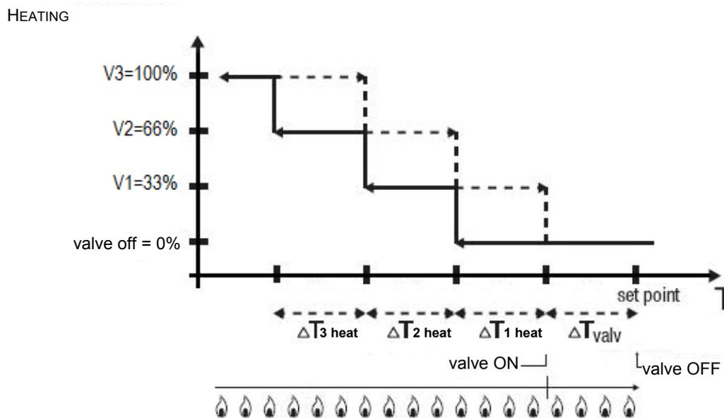
The figure refers to the control of the fancoil speeds with three operating stages for heating. The chart shows that each stage has a hysteresis cycle, and each speed is associated with two thresholds that determine the sending of the associated value. The thresholds are determined by values set for the various regulation differentials, and can be summarised as follows:
