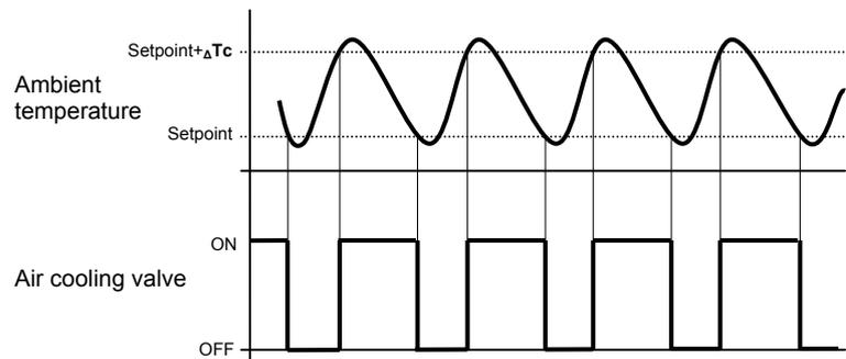
When the measured temperature is higher than the value “setpoint+  $\Delta T_c$ ” (where  $\Delta T_c$  identifies the air cooling regulation differential) the device turns on the air cooling system, sending the relative BUS command to the actuator that manages it; when the detected temperature reaches the fixed setpoint value, the device turns off the air cooling system, sending the relative BUS command to the BUS that manages it.
