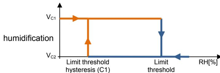
When the relative humidity of reference is lower than value C1 (limit threshold hysteresis”), the device will sent the command associated with Condition 1; when the relative humidity of reference reaches value C2 (limit threshold), the device will sent the command associated with Condition 2,.
