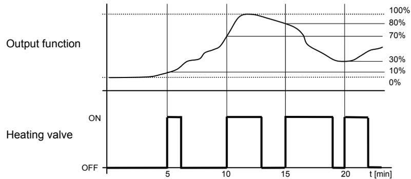
The device keeps the heating system switched on for a cycle time percentage that depends on the output function of the proportional-integral control; the device continuously regulates the heating system, modulating the system turning on-off times with a duty-cycle (shown to the right along the vertical axis) that depends on the output function value calculated at every time interval equal to the cycle time. The cycle time is reinitialised every time the reference set-point is modified.
