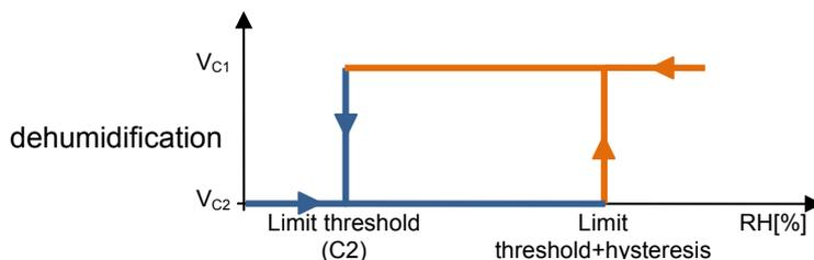
When the relative humidity of reference is higher than value C1 (limit threshold+hysteresis”), the device will sent the command associated with Condition 1; when the relative humidity of reference reaches value C2 (limit threshold), the device will sent the command associated with Condition 2,.
