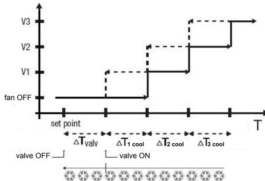
The figure refers to the control of the speeds of a fancoil with three operating stages for air cooling. The chart shows that each stage has a hysteresis cycle, and each speed is associated with two thresholds that determine its activation and deactivation. The thresholds are determined by values set for the various regulation differentials, and can be summarised as follows:
