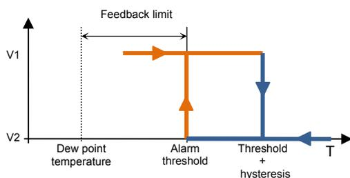
The purpose of the feedback limit is to identify the approach of the dew point temperature, defining when prior to reaching the dew point temperature the command associated to the dew point temperature alarm must be sent. The initial value of the limit is defined via the parameter “**Alarm feedback limit [tenths of °C]**”, which can assume the following values:
