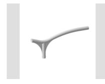
Single pole head bracket in hot galvanised steel tubing, 3 or 4mm thick, painted with polyester powder. Supplied with three M8 stainless steel lockscrews for fixing on poles of 60mm diameter.
