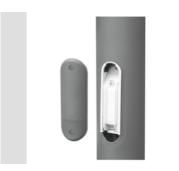
Tapered pole for planting, in 3mm hot galvanised sheet steel painted with polyester powder. With two slots (46x186mm) for cable inlet, and with junction terminal block included. Terminal block door painted in the same colour as the pole.
