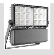
SMART [PRO] 2.0 is a medium power outdoor and indoor LED projector, suitable for lighting sports areas and facilities. It can be installed on the wall, ceiling or ground thanks to the polyester powder coated galvanised steel bracket, with trivalent passivation, equipped with adjustable goniometric scale and supplied in kit. The body is produced in aluminium die casting
