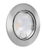
Led decorative recessed luminaire with die-cast aluminum body and adjustable polycarbonate shield, available in white, aluminum, gold and bronze version. Installable on panels with a minimum thickness of 5mm and a maximum of 20mm. Suitable for indoor installation, built-in power supply, IP20 protection degree and good impact resistance.
