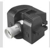
Removable polyamide case containing electrical components , equipped with handle to facilitate the operation time. Two poles power supply terminal in double insulation for max. 2.5 mm² cable. Ceramic lamp-holder. Rigid wiring cables 1-1.5 mm² in silicone with double insulation UG4G4.
