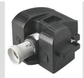
Removable polyamide case containing electrical components , equipped with handle to facilitate the operation time. Two poles power supply terminal in double insulation for max. 2.5 mm² cable. Ceramic lamp-holder. Flexible wiring cables 1-1.5 mm² in silicone with double insulation FG4G4.
