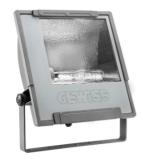
Floodlight in die cast aluminum with galvanized bracket and painted the same color as the body. Equipped with graduate scale to facilitate orientation. Flat tempered glass 4 mm thickness silk screen printed; hinged to the body for quick access inside the Floodlight. Anti aging silicone gasket. Power input through PG13.5 for cables Ø 6.5 ÷ 13 mm. Optic in 99.85% polished and anodised aluminium. Electrical componenent plate in galvanized steel. Quick wiring tripolar terminal block.
