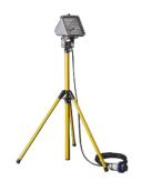
Multifunctional floodlights in die-cast aluminium, painted with polyester powders, for portable applications on adjustable telescopic support (min. 1m - max. 1,4m). Optic in 99.85% polished and anodised aluminium. Flat tempered glass 5mm thickness. Anti-aging silicone gasket. Equipped with protective wire guard and cable type H07RN-F section 3x1,5mm² lenght 5m with plug IEC 309 2P+E 200-250V IP67.
