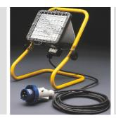
Multifunctional floodlights in die-cast aluminium, painted with polyester powders, for portable applications on tubular support Optic in 99.85% polished and anodised aluminium Flat tempered glass 5mm thickness Antiaging silicone gasket Suitable for use with halogen lamps Equipped with protective wire guard and cable type H07RN-F section 3x1,5mm² lenght 5m with plug IEC 309 2P+E 200-250V IP67
