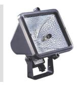
Multifunctional floodlights in die-cast aluminium, painted with polyester powders, for fixed applications. Optic in 99.85% polished and anodised aluminium. Flat tempered glass 5mm thickness. Anti-aging silicone gasket. Suitable for use with halogen lamps. Power input through cable gland for cable Ø 9÷12 mm.
