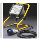
Multifunctional floodlights in die-cast aluminium, painted with polyester powders, for portable applications on tubular support Optic in 99.85% polished and anodised aluminium Flat tempered glass 5mm thickness Antiaging silicone gasket Suitable for use with halogen lamps Equipped with protective wire guard and cable type H07RN-F section 3x1,5mm² lenght 5m with plug IEC 309 2P+E 200-250V IP67
