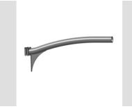
Bracket for fixing on poles of 60-75mm diameter, in hot galvanised steel tubing, 3mm thick, painted with polyester powder. Stainless steel screws and nuts.
