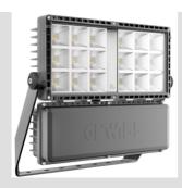
SMART [PRO] 2.0 is a medium power outdoor and indoor LED projector, suitable for lighting sports areas and facilities. It can be installed on the wall, ceiling or ground thanks to the polyester powder coated galvanised steel bracket, with trivalent passivation, equipped with adjustable goniometric scale and supplied in kit. The body is produced in aluminium die casting
