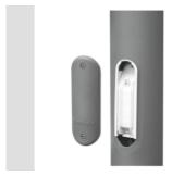
Tapered pole for planting, in 3mm hot galvanised sheet steel painted with polyester powder. With two slots (46x186mm) for cable inlet, and with junction terminal block included. Terminal block door painted in the same colour as the pole.
