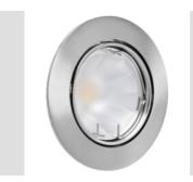
Led decorative recessed luminaire with die-cast aluminum body and adjustable polycarbonate shield, available in white, aluminum, gold and bronze version. Installable on panels with a minimum thickness of 5mm and a maximum of 20mm. Suitable for indoor installation, built-in power supply, IP20 protection degree and good impact resistance.
