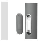
Tapered pole for planting, in 3mm hot galvanised sheet steel painted with polyester powder. With two slots (46x186mm) for cable inlet, and with junction terminal block included. Terminal block door painted in the same colour as the pole.
