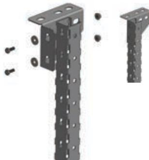
Light ceiling support secured with M6 screws (Maximum torque: 10 daN.m for max. length 500 mm)
