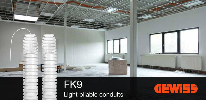
FK9 is a new light pliable conduit made of PVC with a compression resistance of 320 N and impact resistance of 1 J at -5 °C, classified 22212. FK9 is recommended for installation in chased wall or ceiling and represents the best solution for those who do not require an high impact resistance but at the same time do not want to compromise on quality.
