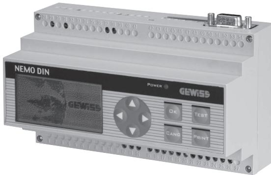
The **NEMO DIN PLUS** module is housed in a 9 modular container with a DIN rail. It is supplied with 4 LON lines RS485 (39 Kb/s) required for communication with the Gewiss STARTEC NET emergency lamps. The user interface is implemented with an O-LED display and a membrane keyboard. The **NEMO DIN PLUS** module offers all the functions required for:
