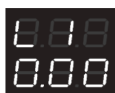
Instantaneous absorption of load 1 available, load ON and absorption 0W
