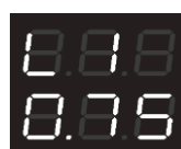
Instantaneous absorption of load 1 available, load ON and absorption 750W
