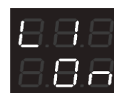
Instantaneous absorption of load 1 not available, load ON
