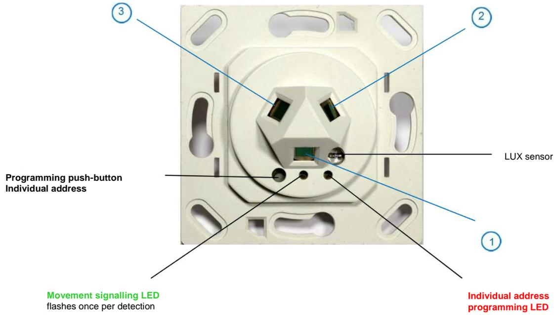
Fig. 9.2: location of the three PYR sensors in the device
