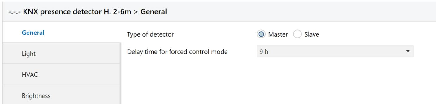
Fig. 3.1: Menu with Type of detector - Master
