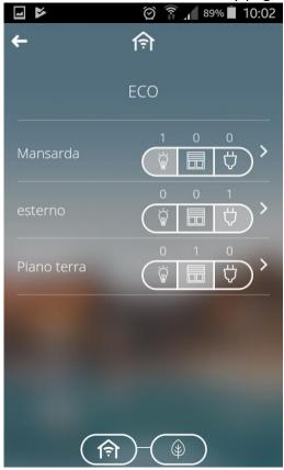
For each zone and environment, the ECO page shows all the circuits that are currently active in the system, with the possibility of sending a deactivation command to each one. The page is dynamic, and only zones/environments with at least one active circuit are shown.
