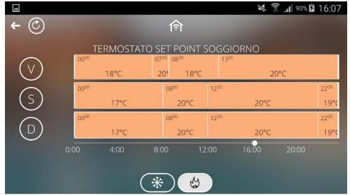
There are two push-buttons at the bottom of the screen which let you view and modify (if necessary) the profile of the heating system and that of the cooling system; in fact, two separate profiles are reserved for each channel for the two types of operation. The Smart Gateway sends the correct commands based on the type of operation active on the controlled device.
