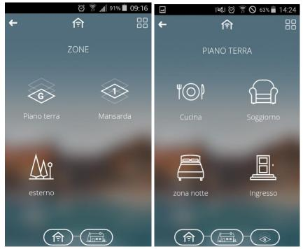
The **Zones/Environments** view lets the user navigate the system using the topology of the house or building programmed during the configuration.
