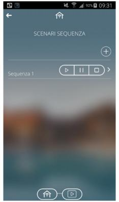
A scene sequence can group together a series of commands to the devices in the field, with the possibility to delay their implementation; the Smart Gateway manages the implementation according to the settings configured. The main page shows a list of the sequence scenes available with the relative commands:
