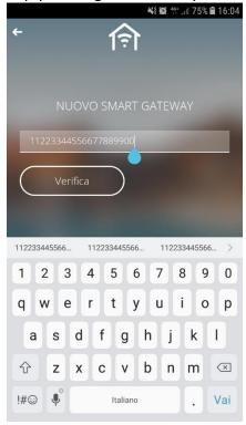
In order to create a new system, you will be asked to enter the ID of your GEWISS IoT device; the identification code is shown on the label on the device itself (see the Smart Gateway example below)
