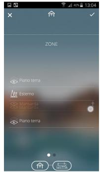
Touch and drag the element to the required position; at the end of the operation, click on the "V" symbol in the top right of the screen to confirm the modification or click on "X" in the top left of the screen to cancel the modification.
