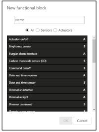
Apart from the name of the functional block model, the right-hand part also shows the category: Actuator (A) or Sensor (S).
