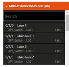
A complete list of the addresses, in ascending order (visualisation at three levels). For each address, you can see the name, size and Data Point Type (if specified in ETS).
