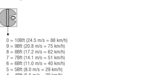
After exiting test mode, wait for 4 seconds for the device to correctly read the selected wind speed.
