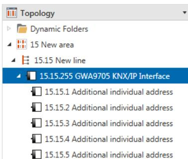
Each address can be modified by entering the required value in the **Individual Address** field of the **Properties** window; if the field frame turns red, this means the address is already being used in the ETS project.
