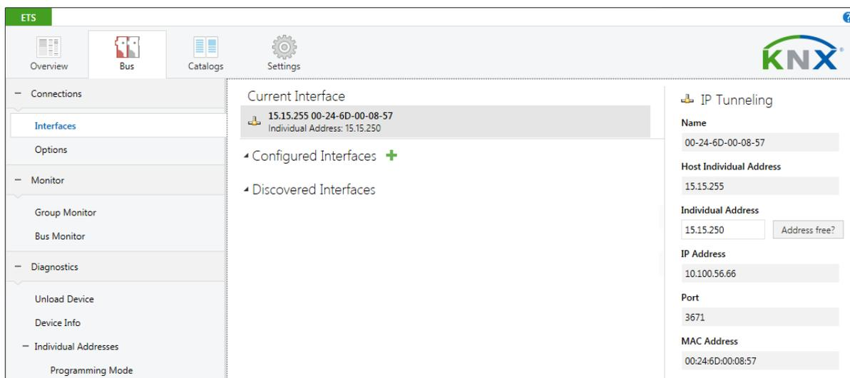
The physical address of the device, and the additional physical addresses, can be modified within the ETS project once the device has been inserted in the project.
