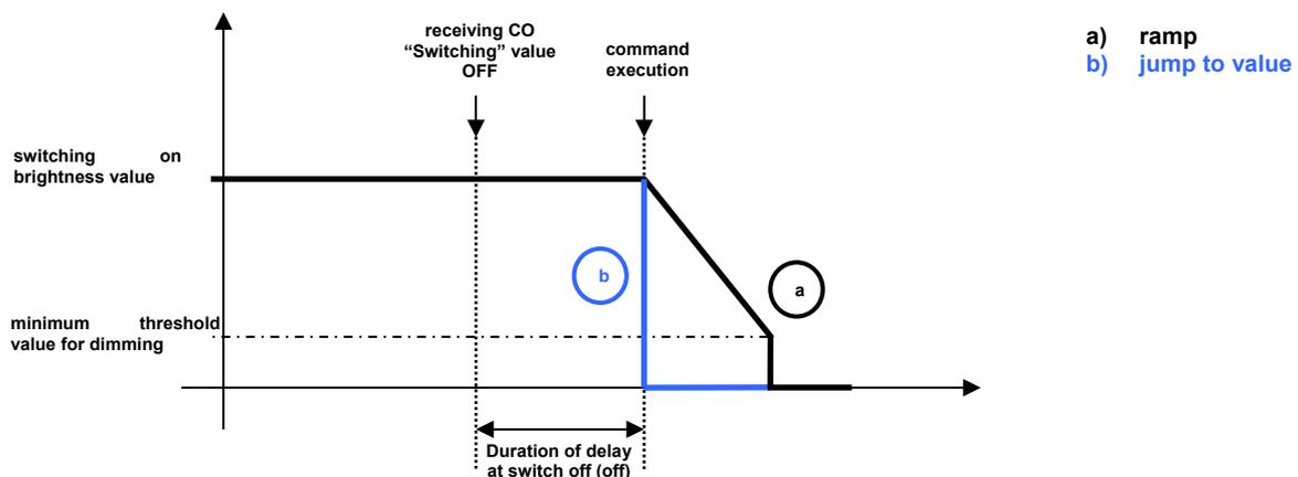
If selecting the **double step** value, the switching off phase is divided into two steps. When an off command is received, the jump to value 0% (0) or the start of a down ramp are delayed by 50% of the
