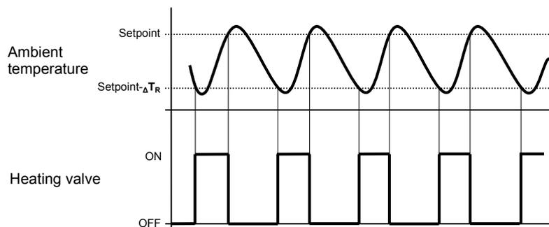
When the measured temperature is lower than the value  $\text{setpoint} - \Delta T_R$  (where  $\Delta T_R$  identifies the value of the heating regulation differential) the device turns on the heating system, sending the relative BUS command to the actuator that manages it; when the detected temperature reaches the fixed setpoint value, the device turns off the heating system, sending the relative BUS command to the BUS that manages it.
