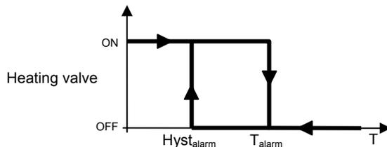
The parameter “**Temperature alarm hysteresis (tenth of °C)**” is used to set the hysteresis threshold of the floor temperature alarm that, subtracted from the temperature alarm threshold, determines the value under which the heating system is reactivated. The values that can be set are:
