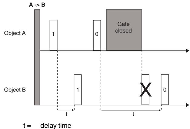
**Example 2:** The gate is closed and the delay time is active. The time has elapsed and the gate is still closed. If the gate is opened, an output telegram will be sent immediately.
