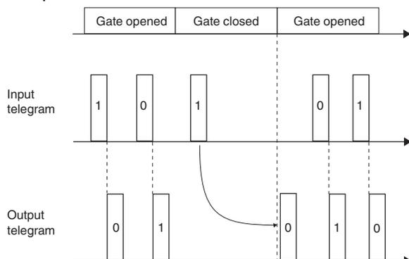
Setting: The gate closes, the last telegram is saved. The status of the output is inverted. The gate is opened again and the saved telegram is forwarded with inverted value (1 -> 0).
