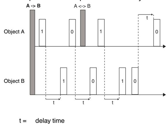
Example 3: The previous telegram is deleted following the change of direction to **B / A**, as the multiplexer block is deactivated.
