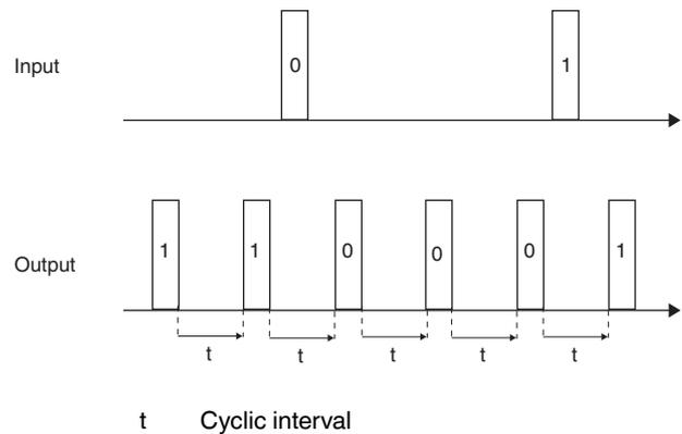
**Cyclically and output change:** In addition to the cyclical sending, output telegrams will also be sent in the case of changes at the input. The send conditions for output telegrams outside the cyclic interval result from the definition of send criteria (output change or receipt of a telegram). This setting is wise if cyclical telegrams and a rapid response are expected (e.g. weather alarm at the blind actuator).
