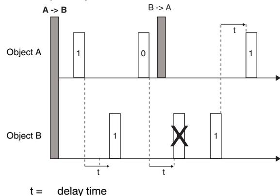
Example 2: The previous telegram is sent to the bus following the change of direction to **A <-> B**. Both objects are the input and the output simultaneously.
