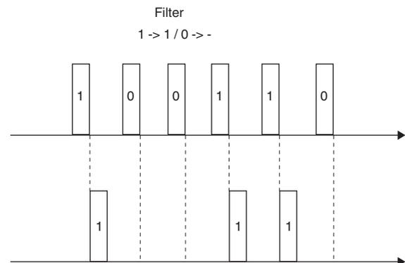
Example 2: **1 -> - / 0 -> 1.** 1 telegrams are filtered out and 0 telegrams are converted into 1 telegrams.
