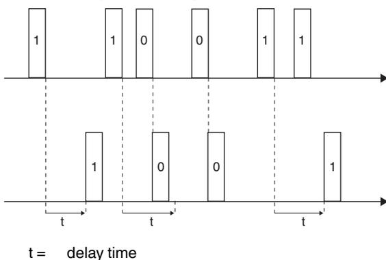
Example: **Time delay if 0 and 1.** Both telegrams are forwarded with a time delay.
