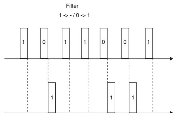
Example 3: 1 -> toggle / 0 -> -. 0telegrams are filtered out. The 1 telegrams toggle between 0 and 1.
