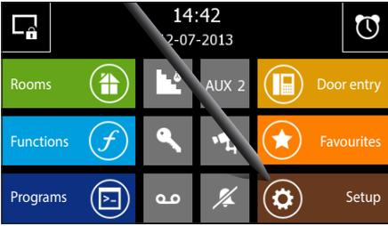
By selecting the "Setup" button from the main page you access the screen that brings together all the settings that involve the overall operation of the panel.
