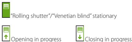
If the system's configuration allows it, the percentage the "Rolling Shutter"/"Venetian blind" is open can be read on the button.
