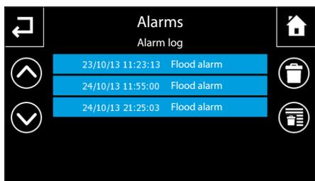
*Note: The melody, rings and volume of the ringtone associated to all the alarms is managed from the "Setup" menu. The acoustic signal is repeated every minute until it is silenced or the alarm condition ends.*
