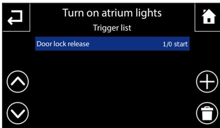
By pressing directly on one of the inputs on the list, you again access the page on which it is possible to choose the action associated to the value that the selected input can take on.
