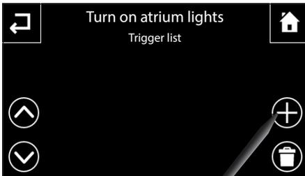
By pressing button and then button , it is possible to select inputs that can recall/stop the "Scenario sequence".
