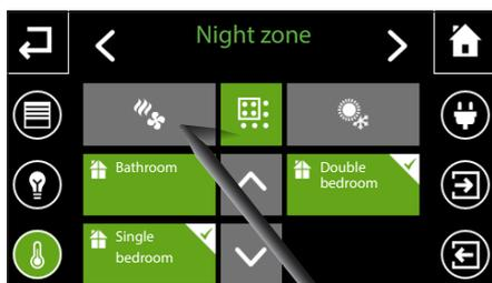
With the "Temperature regulation" filter active, press button (multiple selection) and select the rooms in which the devices to be commanded are.
