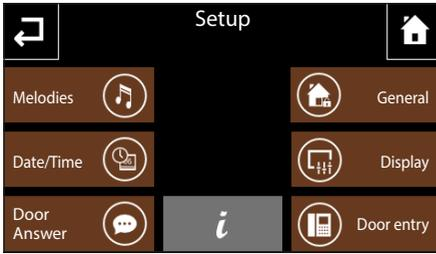
Press on the "Display" button to access a screen that lets you adjust the brightness of the display.
