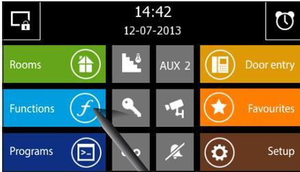
By selecting the button "Functions" on the main page you access the screen that lets you see the "Functions": KNX Scenes, Burglar alarm, Irrigation, Energy data, Loads control, Alarms.
