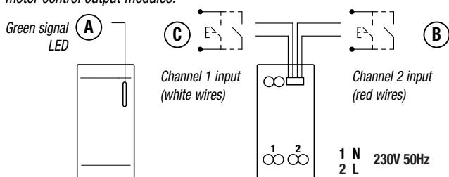
The module is provided with a green signal LED (A). The two inputs (B-C) are dedicated to the connection of contacts, without potential, of control appliances (buttons, switches, sensors, etc.). The module is powered at 230 V.
