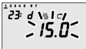
Press key to activate the function, the symbol appears on the display while the value of the set point active at that time starts blinking. Use keys to set the new value of the temperature set point. Use keys to set the number of hours of activation, that will be displayed on the display. Press key , or wait 5 seconds to confirm the setting made.
