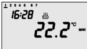
In **manual operation** the timer-thermostat permanently uses a temperature set point that can be freely set. The text MAN and the ambient temperature measured appear on the display.
