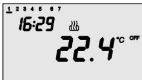
**Antifreeze operation** is only active in heating. In this case the timer-thermostat uses the set point of the antifreeze temperature set. The text OFF and the ambient temperature measured appear on the display.
