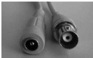
The telecamera has a Y cable, about 35cm long, fitted with a female BNC connector at one end for connection to the video signal, and a male coaxial plug (internal  $\varnothing$  2.1mm, external  $\varnothing$  5.5mm, length 11mm - positive at centre) for the 12V DC power supply.
