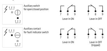
NOTE: to change the function Aux contact 2, from open/closed position to fault indicator switch and viceversa, it's required to turn the selector by screwdriver and to make an automatic reclosing cycle.
