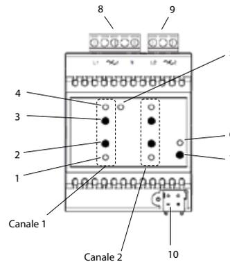
1. LED signalling the type of load
