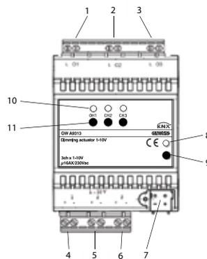
1. Screw terminals for the relay contacts of the power supply to ballast, channel 1
