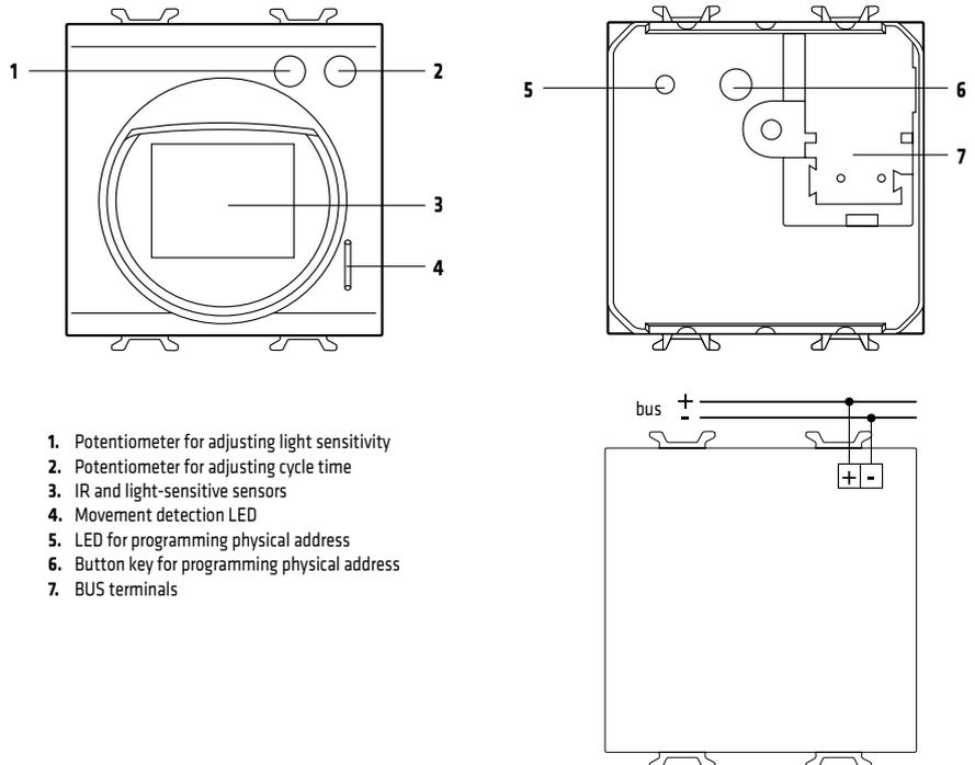
1. Potentiometer for adjusting light sensitivity
