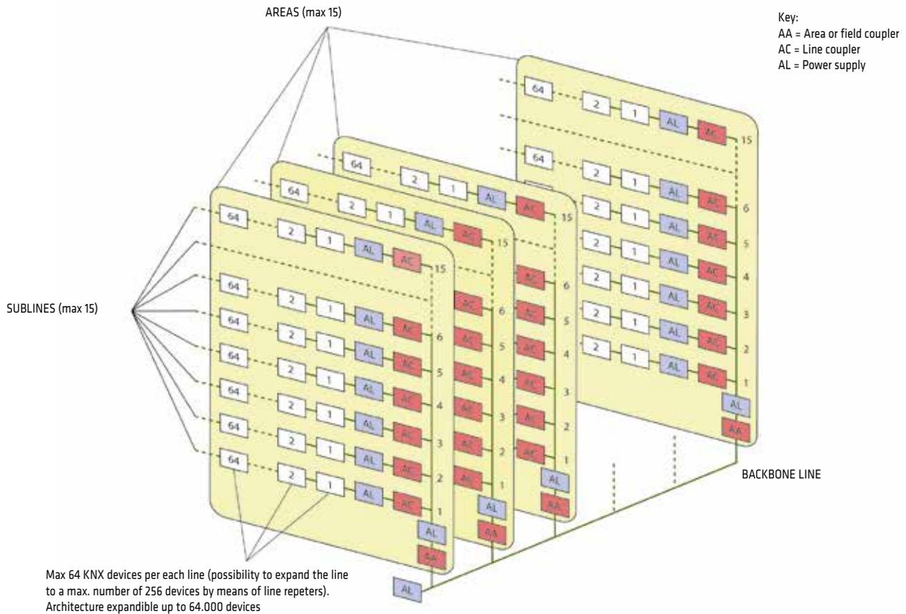
The Main Area Lines are connected to the Main Backbone Line through special devices called Area (or Field) Couplers, while the Sublines are connected to the Main Lines through Line Couplers.
