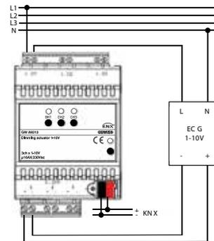
5. Screw terminals for the control voltage 1-10V canale 2
