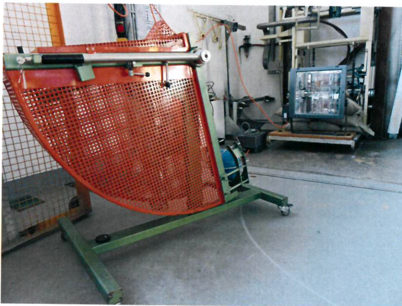
Picture 2: Luminaire fixed with bracket (right) and ball throwing machine (left)
