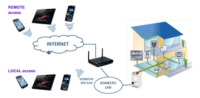
The KNX/IP interface is connected (via cable) to the home network through the modem-router.
