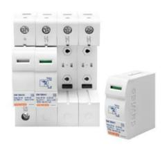
maintenance easier. The optical indicator on the front changes from green to red to show that the device has reached the end of its lifespan. Thanks to the integrated auxiliary contact, it is possible to immediately report the inefficiency of the protective device. The removable cartridges make replacement easier and quicker, and prevent wiring errors.
