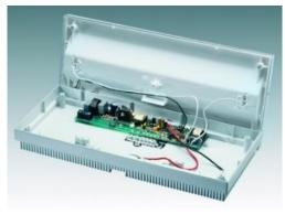
All the luminaires are equipped with a double internal microprocessor: one for managing the lamp and performing the self-diagnosis tests, and the other for managing communication with the NEMO DIN PLUS system control unit.
