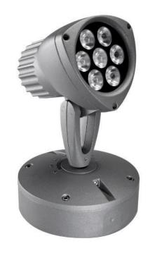
The floodlights can be freely orientated on their two axes, and are equipped with a pointer that defines the degrees of tilt. In the case of white light, DMX management lets you choose different levels of light intensity and transitions for each single floodlight. The colour management control unit has a LED display with icon navigation, and can command up to 20 LED RGB Dedalo or Saturno devices via the DMX protocol.
