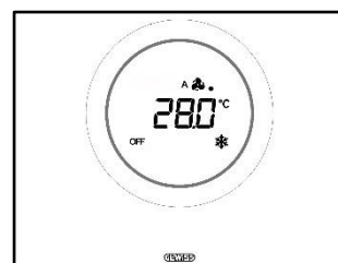
HVAC – OFF Răcire
